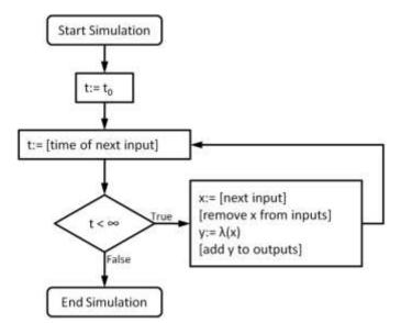
Figure 2: Simulation procedure for Formalism A.
