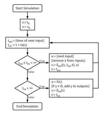
Figure 4: Discrete event simulation procedure using DEVS.
