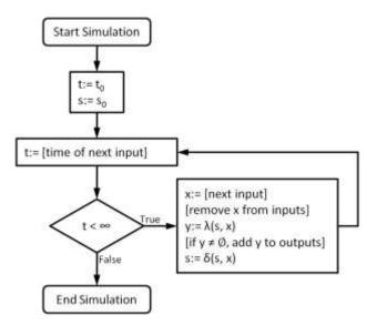
Figure 3: Formalism B Simulation Procedure.
