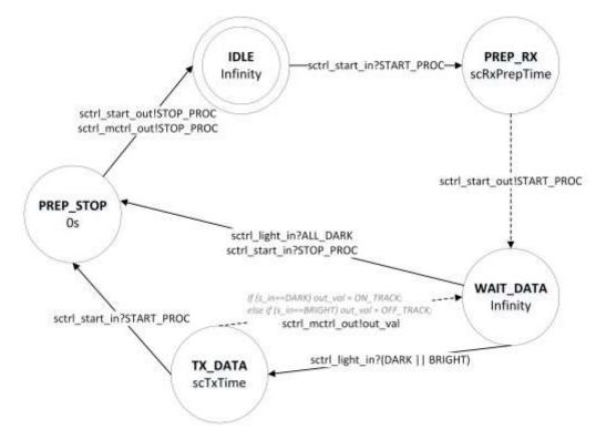
Figure 5: Sensor controller state diagram.
